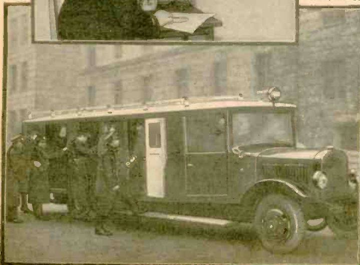
Left—Special giant, loop-type, short-wave receiver in use by Vienna police expert for listening in on "unlawful" radio transmissions. Above—portable short-wave, loop receiver used for listening in on unlawful transmitters. Right—radio truck of the Vienna police fitted with radio cabin and aerial on the roof.
