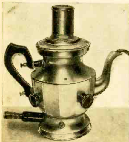
Here we have a close-up view of the "coffee-percolator" 2-tube receiver, which has brought in world-wide S-W stations from many foreign climes.
