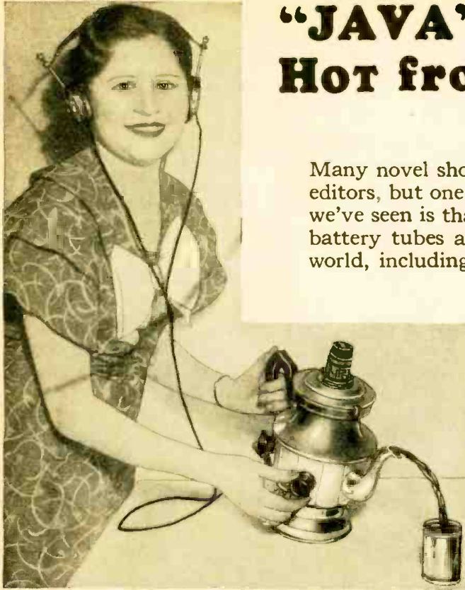
Left—The young lady is pouring out some hot jazz from Java. The tuning and regeneration control of the set built within the percolator are adjusted by means of the external knobs shown. Battery current for the tubes is taken in to the set through the wires passing through the spout.
